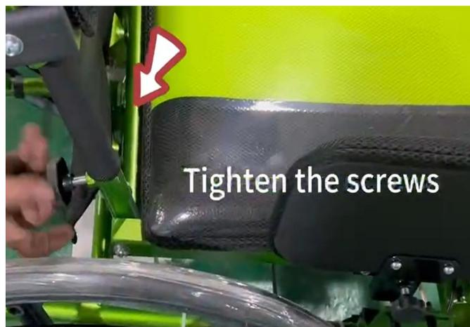
**7.1.4 Loosen the screw first, then insert the handle and tighten the screws.**
